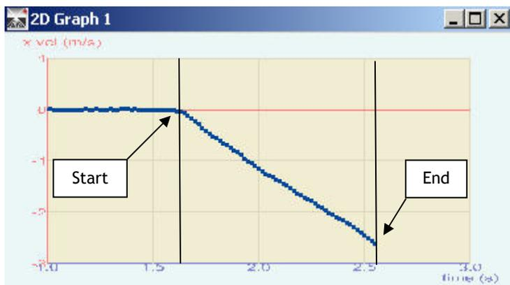
$$\text{X Acceleration} = \frac{(V_{X_f} - V_{X_s})}{\Delta \text{ Time}}$$
