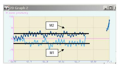
When the 200 gram hanging mass is released, it supplies the force that accelerates the 100 gram hanging mass. If friction effects and the masses of the string and pulley are ignored, then the approximate average acceleration of the system is given by the above graph.
