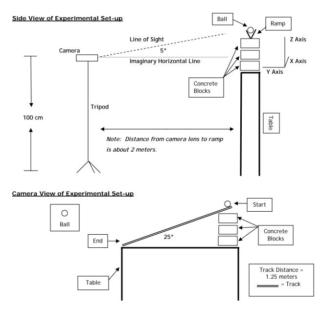
In this activity, the ball moved leftward and down the track. Since the motion of the ball occurs both in the horizontal and vertical directions, the video camera settings must be modified. This can be done by choosing *2D Camera Alignment* under the *Experiment* menu item [Figure 1.]
